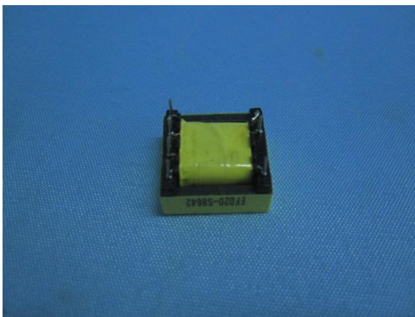
High frequency transformer
